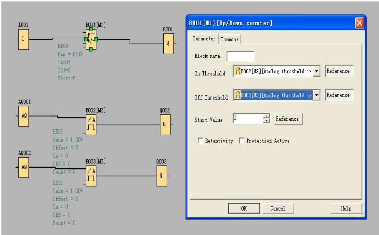
Set AQ1 (the address configured in the below figure is for economic/ standard ELC-18) value via ELC-MD204L( AQ also can be replaced by AF in above figure)
