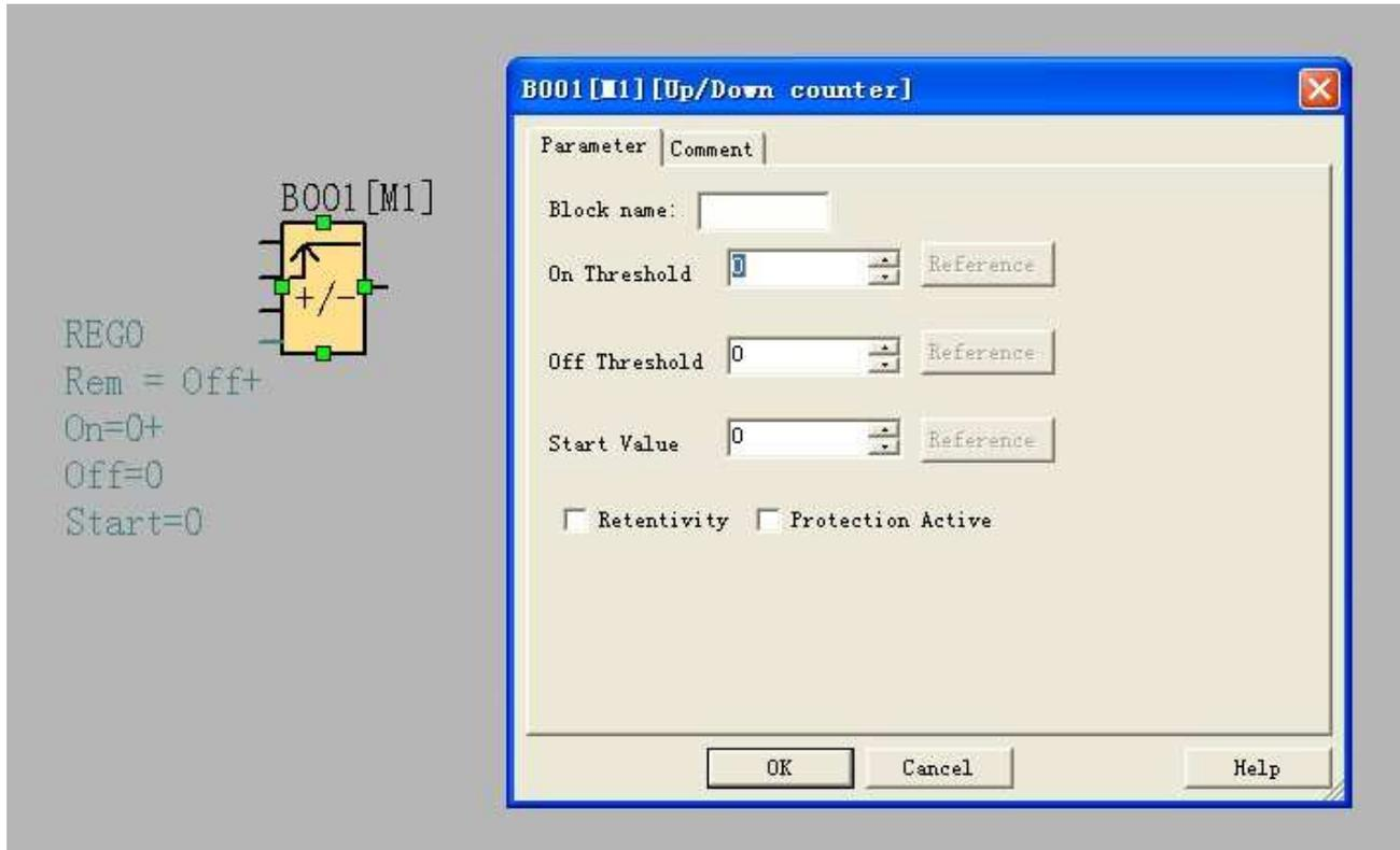
The REG0 value is to show the current counter value of the block (B001) ,it's not the value of "On Threshold"/"Off Threshold".
