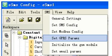
Configure the APN based on your SIM card and then click "Write" to download the configuration into x-Messenger.
