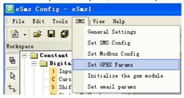
Configure the APN based on your SIM card and then click "Write" to download the configuration into x-Messenger.
